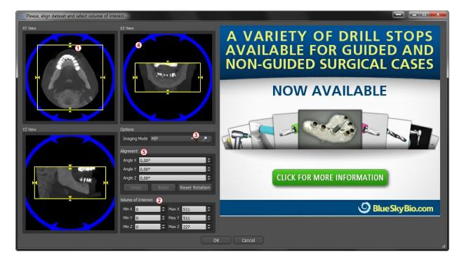
The data can be aligned using the blue circles (4); it is also possible to enter values for rotation around the individual coordinate axes manually (5). The transformation performed then applies correctly for importing and exporting data as well.
